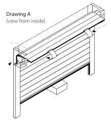
v. Position unattached end of locking/attachment arm so that the fixing bar lines up with locating holes in the two collars (rotate axle with override if necessary) and slide collars together making sure pre-positioned collar is tight against rivet – see Drawings B & C
