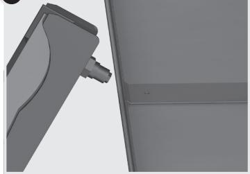
Drill a hole with a 4.2mm drill bit through this hole and the fascia.
