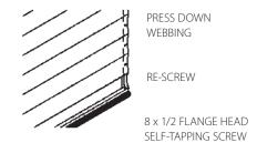
iv. If the number of slats has been reduced, trim the webbing accordingly and carefully melt the cut ends to prevent fraying.
