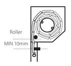
N.B. To prevent damage to the motor make sure the door is stopped by reaching the limit switch. Do not allow stops to come into contact with guide rollers.
