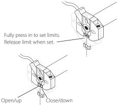
**Left Hand Motor:** Fully press in limit switch to activate. Press and release switch when door has been set to stop in correct position. The yellow limit switch activates the OPEN/UP limit. The white limit switch activates the CLOSE/DOWN limit.
